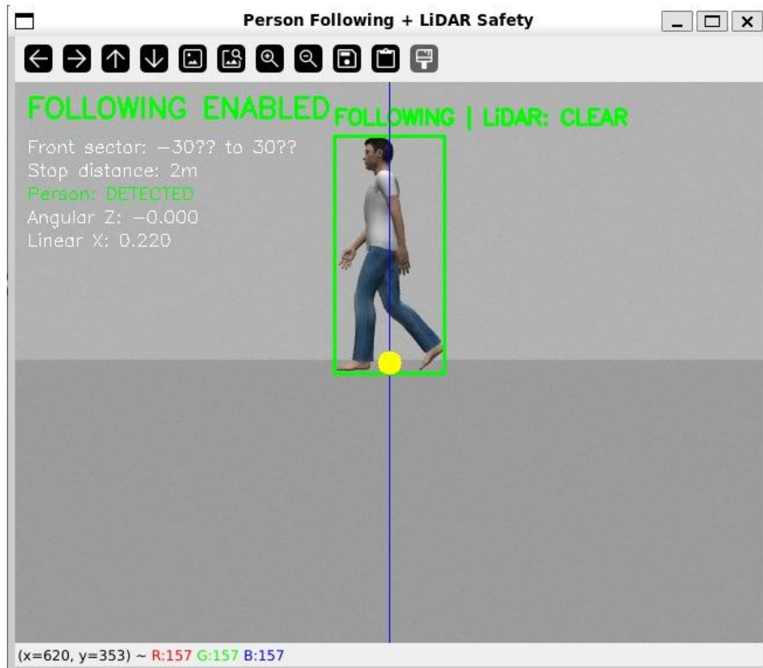
Fig. 7.1 Camera-based person detection and following enabled in Gazebo environment
